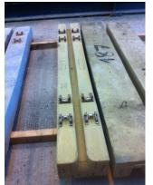
CEMEX Rail solutions at Washwood Heath have just started production of a G55 Cable Management Sleeper. This sleeper range provides a solution for getting cables for signalling and telecommunications safely across the track.
