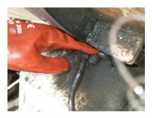
In a recent incident a truck mixer driver, working for an Independent Haulage Contractor, was lucky to escape more serious injury when he decided to grease the moving track ring of his drum with his gloved hand. His finger was trapped by the drum locking mechanism, resulting in the loss of his finger tip.
