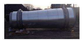
The Dryer at Fridaythorpe drum mix plant was worn out and causing issues on a daily basis up to the point that the plant had become the most unreliable plant in the UK. When the Team did the budgets last year they planned to replace the dryer as part of the maintenance plan. Rather than just replacing the dryer, the drive system was upgraded with high efficiency geared motor units driving the roller paths. The benefit to this design is it reduces energy consumption,
