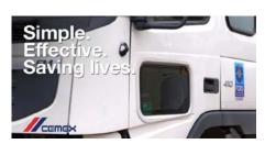
A new simple and effective safety measure, a door with a 'window' or the Vision door will help CEMEX drivers have better nearside vision for seeing vulnerable road users. The new measure, a simple glass panel fitted in to the bottom half of the nearside door, allows the driver to see the head and shoulders of anyone passing close to the vehicle.
