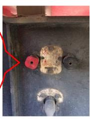
The trailers park brake (Red Button) should be pulled out when the trailer is left unattended and detached from the tractor unit.
