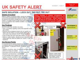
Isolation of machinery before carrying out maintenance is one of the most fundamental health and safety rules. Recent fatal incidents in the industry, including one in our own operations, have illustrated the tragic consequences when isolation is not 100% effective.
