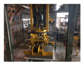
Over the past couple of years Buxton Block Plant has been struggling with packing blocks due to the old cube grabs - these grabs take the blocks off the production line and stack them up before being banded together. They are the original parts of the machine and were causing many hours downtime over each week despite the best efforts of the maintenance team. They were also costing us valuable production time.
