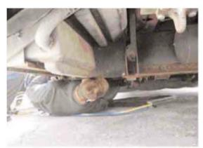
Vehicle ground clearance can suddenly and unexpectedly change due to a drop-in air pressure. This presents crushing and trapping hazards to technicians repairing vehicles, especially if working beneath them. There is also a risk of trapping around the wheel arch.
