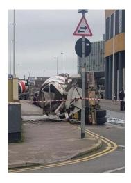
There has been a worrying trend across Europe including the UK, of vehicle rollovers. A truckmixer in the UK operated by an independent haulage contractor, rolled over whilst on route to a customer site. The incident occurred as the vehicle entered a sweeping right-hand bend and resulted in the vehicle turning onto its nearside, coming to rest partially on the pavement and on the public highway.
