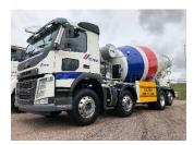
Midlands-based concrete mixer supplier, Hymix, has redesigned the Readymix Concrete Mixer taking away the need for the ladder and platform thus removing the necessity for the driver to work at height, helping to ensure his or her safety. This is just one of the latest innovations focusing on pedestrian, cyclist and driver safety launched by Hymix at 'The 2019 Concrete Show' on 20<sup>th</sup> and 21<sup>st</sup> March at the NEC, Birmingham.
