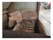
In the UK, we did, however, suffer a High Potential (HIPO) incident on one of our plants, where a ground receiving hopper collapsed and fell in to the pit (pictured).
