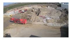
Dagenham Wharf crushing has started! We will be recycling approximately 12,000t of returned concrete waste into a sand and graded stone which will all be used internally by Readymix. A huge cost saving and benefit to the environment.
