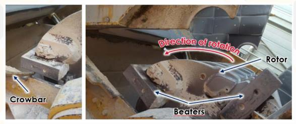
In the morning of the 3rd day of the operation, in order to replace the last 2 beaters, the team applies the operating mode: the rotor is released then starts to rotate very slowly and is going to stop.
