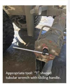
CEMEX was acting as principal contractor on a Soil Stabilization contract and had sub contracted this work to a third party. The accident took place on a rural road, about 5 kms from the contract site, when the worker was checking the cement spreader equipment and trying to unblock the screw conveyor located at the rear. He was pulling a homemade wrench towards him, which slipped off and hit his face, causing a cut to his face. Both vehicle and screw were switched off.
