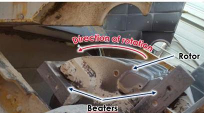
In the morning of the 3rd day of the operation, in order to replace the last 2 beaters, the team applies the operating mode: the rotor is released then starts to rotate very slowly and is going to stop.
