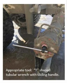
CEMEX was acting as principal contractor on a Soil Stabilization contract and had sub contracted this work to a third party. The accident took place on a rural road, about 5 kms from the contract site, when the worker was checking the cement spreader equipment and trying to unblock the screw conveyor located at the rear. He was pulling a homemade wrench towards him, which slipped off and hit his face, causing a cut to his face.
