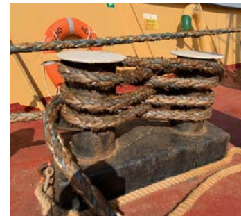
Rope turns riding up Bitts under load
