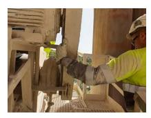
The concerning run of serious injuries across the Region continues, with an incident last week in Spain where an employee suffered severe trauma to four fingers of one hand, when they came in to contact with the drive belts for a conveyor. It seems the employee gripped the guard as he accessed the conveyor walkway, however, there was no protection at the back of the guard.
