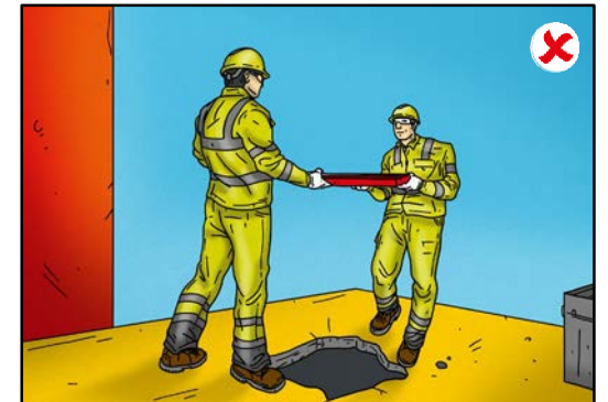
Not secured workplace
