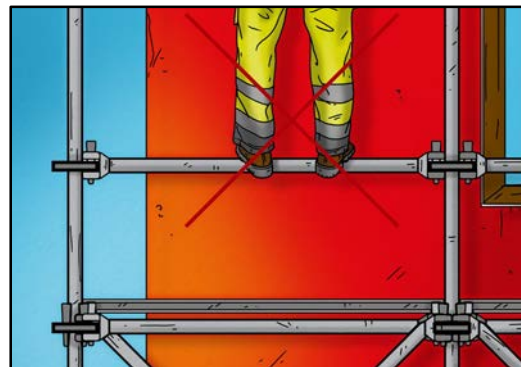
Do not raise the work site by using unstable objects or by using the scaffolding construction.
