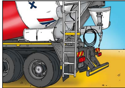
If they cannot be accessed from the platform, safe access to the vehicle must be ensured.
