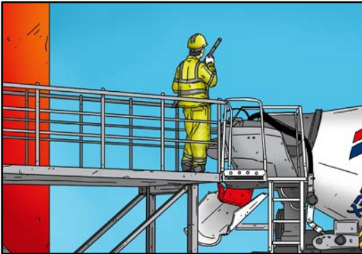
There are fixed or mobile platforms for safe access to trucks.
