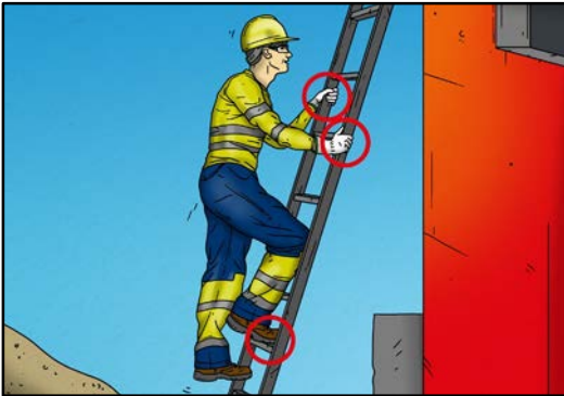
Always use three contact points when climbing up or down a ladder.
