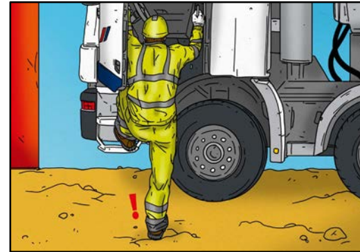
When entering and exiting the vehicle use three points of contact and face the vehicle. (Be careful when descending onto an uneven surface.)
