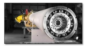
A new burner pipe is being installed during the kiln shutdown. This is a Unitherm burner which is proving highly successful across CEMEX to increase alternative fuel burning at the front end of the kiln.
