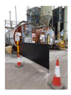
As part of continual efforts to improve the Health & Safety on site, the team at Preston Asphalt plant have this month fabricated and installed a bitumen splash gate. This provides a safety barrier between discharging bitumen tanker and our collect customers; and very swish it looks too!
