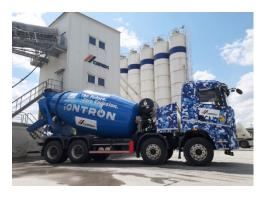
The prototype Putzmeister iONTRON e-Mixer vehicle will be operated for a week from ready-mixed production plants in Pruszków and Warsaw.
