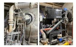
At Salford Rail depot CEMEX has invested in a new second dual fuel burner. This will be more efficient and will lower gas and kerosene usage, further reducing carbon emissions on site.
