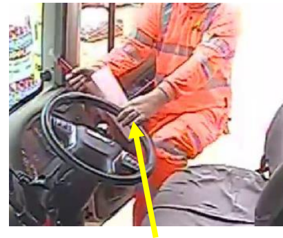
Incorrect handhold for the driver and final landing when driver fell
