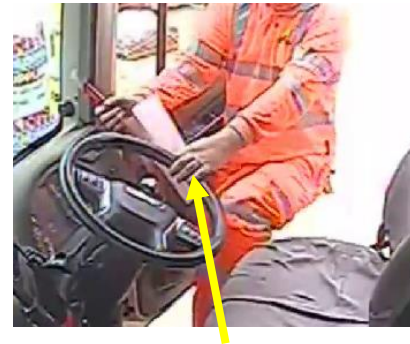
Incorrect handhold for the driver and final landing when driver fell
