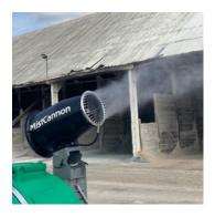
The team at Salford Aggregates plant have recently been trialling a mist cannon to reduce dust on site.
