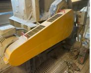
During August, the team at Salford Aggregate Plant made safety improvements to fit new drive guards on rotating shafts, ensuring that any accessible moving parts are covered.
