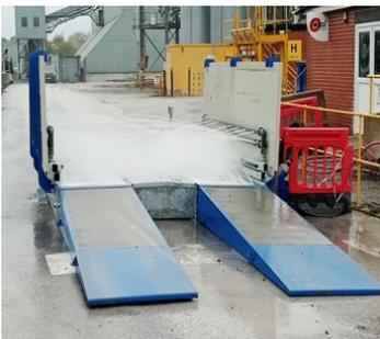
Thank you to the team at Stourton Asphalt plant for sharing their latest Health & Safety improvement. They have installed a new wheel wash before the site’s exit, to eliminate “drag off” onto public roads which has increased due to much higher depot volumes.
