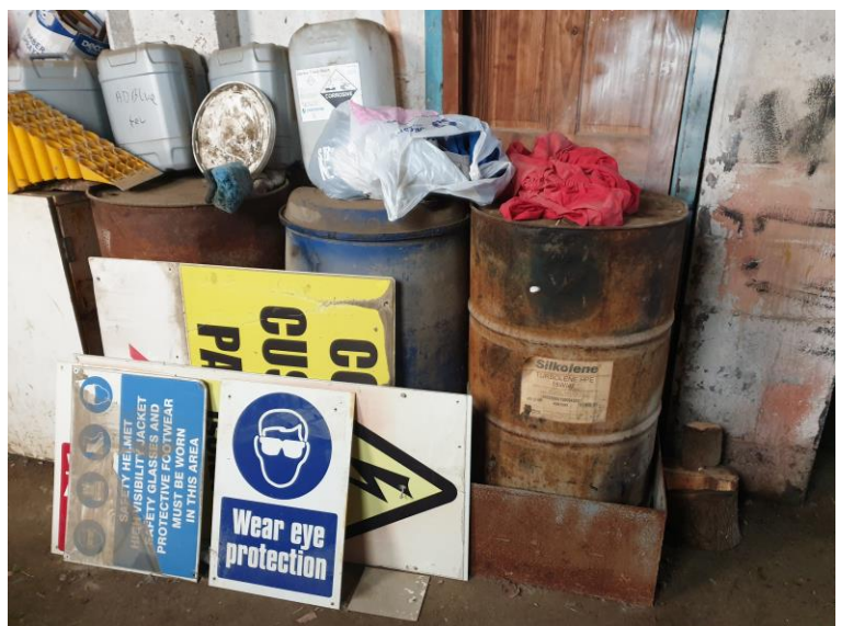
Poor compliance with oil storage regulations and bad housekeeping
