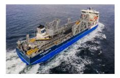
UK Marine's Cemex Go Innovation (CGI) specialises in the extraction of sand and gravel from the seabed. It is designed to extract aggregates from the seabed up to depths of 55 metres. The ship has been developed to offer major environmental savings while ensuring safety, high performance and sustainability.
