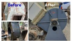
During a recent audit at Preston Asphalt plant it was noted that the guarding around a large fan needed replacing. The fan is used for drying, heating and controlling emissions.
