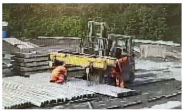
Operator exiting cab forwards without three points of contact
