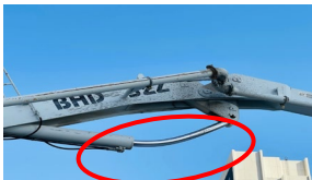
Missing pin caused the bent cylinder
