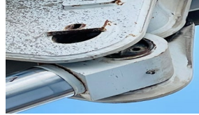
Missing pin caused the bent cylinder
