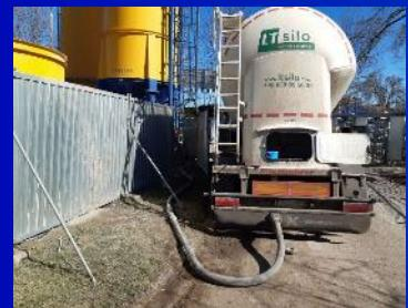
After unloading bulk cement at a customer site, a driver began disconnecting the hoses without realizing compressed air remained in the pipeline. Cement was expelled, dislodging his helmet and goggles and covering his face. He received eye washing as first aid but suffered an allergic reaction from the cement contact.
